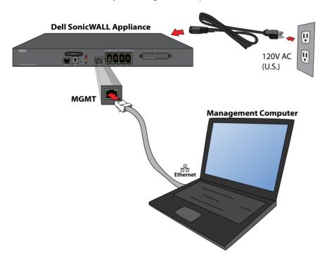
The following sections provide initial configuration information and instructions for connecting your Dell SonicWALL NSA 2600 appliance for initial setup.
